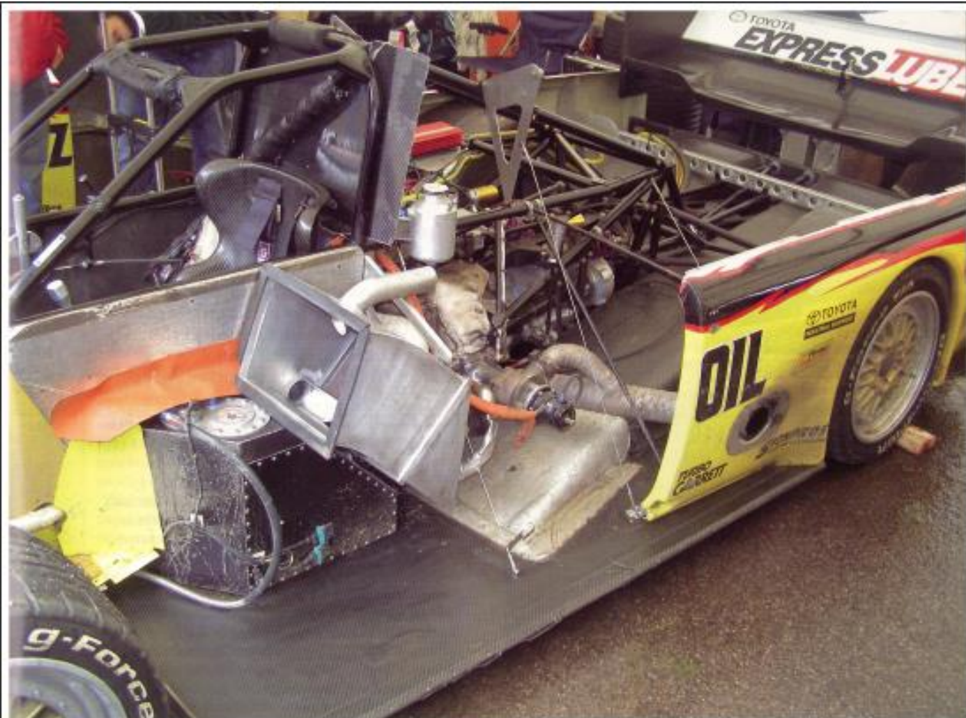
Above: Note tunnels starting each side of engine and ducting for air filter and intercooler either side of driver. Roll cages seems simple for performance of the vehicle!
