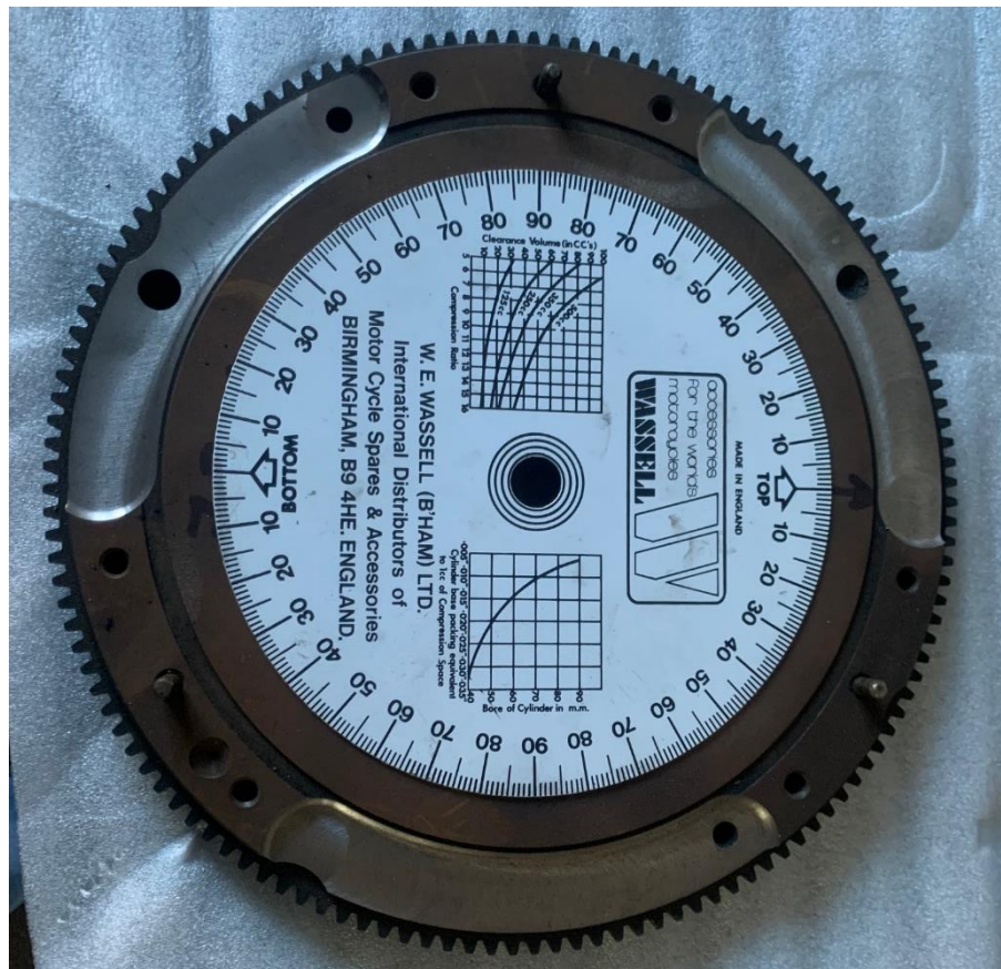
Degree Wheel on a flywheel with double sided tape
