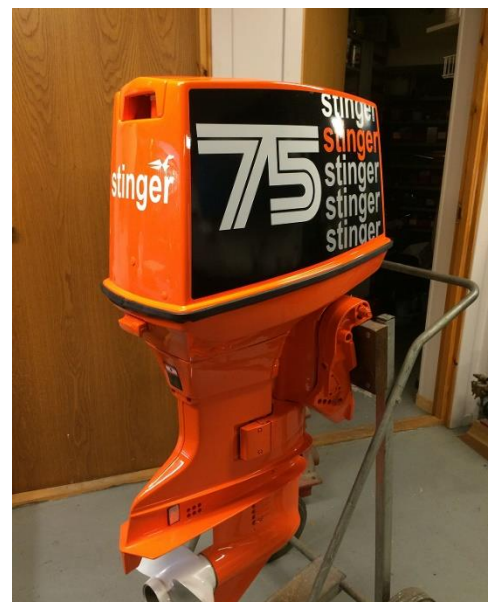
A Johnson 'Stinger' outboard motor from the early 1980s
