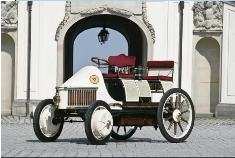
Porsche Semper Vivus recreation, showing the hub motors used in the front wheels.
