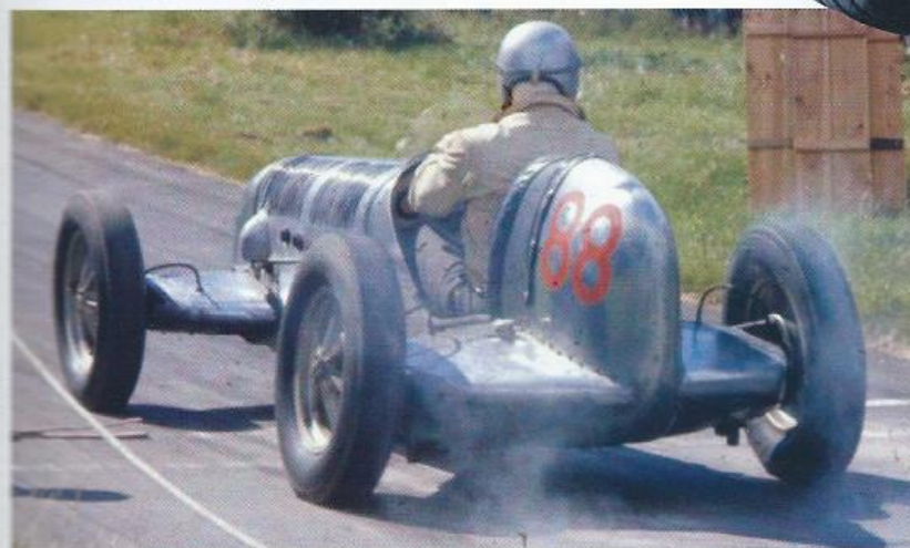
Above: The rudimentary windscreen was soon dispensed with. Note the drilled steering wheel, so painstakingly made by Dowson, and the gearbox with its central change. Below: The Lightweight seen at Prescott hill climb in the 1960s with George Dowson at the wheel
