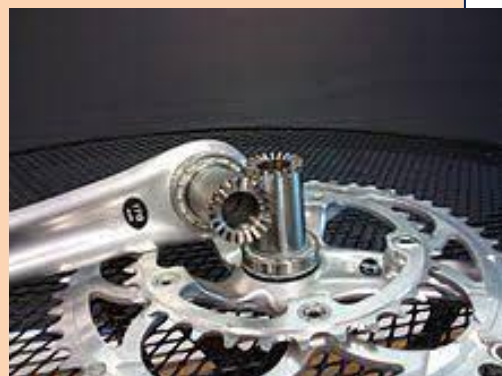
A Hirth joint (coupling) as used to connect a crank to a bottom bracket shaft on a Campagnola bicycle. Source: Wikipedia.com
