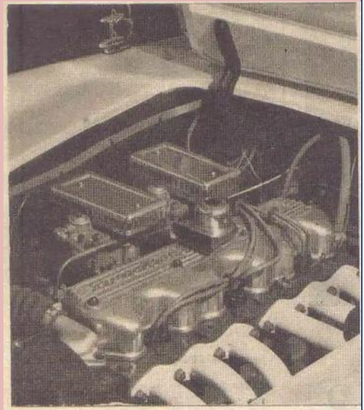
Engine bay of the 'Record' car: Repco 'Hi-Power' headed Holden 'Grey Motor' 2.3 litre OHV 6 cylinder, cross-flow engine fed by 2 Weber carbs. Circa 133 bhp with a 'cooking cam' and extractors. (SCW Magazine)
