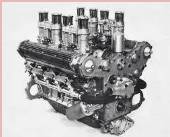
RB620 engine, as used by Team Brabham in Formula 1. Source: primotipo.com
