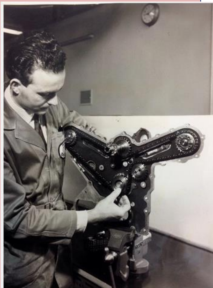
Assembly of chain in the magnesium timing case of an RB620 engine (Repco)
