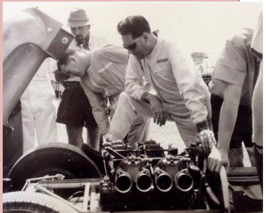
Jack Brabham looking carefully at the Buick 3.9 litre engine in the mid-engined Scarab RE at Sandown Park, Melbourne in 1962, filing the information away for future reference! (Doug Nye with Jack Brabham)
