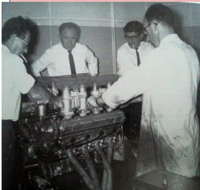
L>R: Phil Irving, Bob Brown, Frank Hallam and Peter Holinger dyno testing the first 2.5 litre Tasman RB620 engine at Russell Manufacturing's engine test lab in Richmond in March 1965. Weber carbs borrowed from Bib Stillwell, the engine did not race in this form. The engine initially produced 235 bhp @ 8200 rpm, equivalent to a 2.5 Coventry Climax engine. 'Ciggies a wonderful period touch (Repco)
