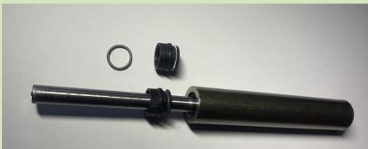
Bill's tool for inserting valve guides into FIAT heads.
