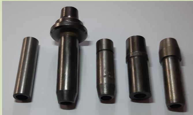
A range of valve guide shapes and sizes, from supplier Automotive Surplus P/L (with thanks)
