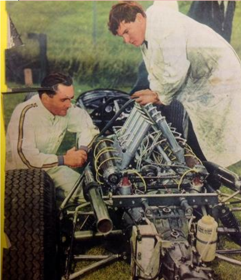
Jack Brabham, Repco engineer Nigel Tait, and Brabham BT19 Repco at Sandown Park Melbourne for its Tasman Series debut, January 1966. RB620 'E2' engine in 2.5 litre capacity. (Australian Post magazine)
