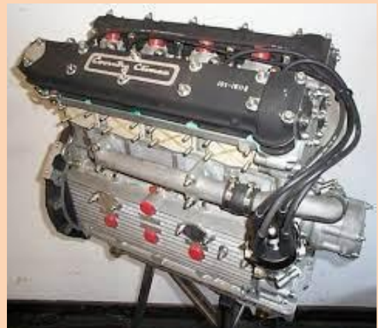
Coventry-Climax 1.5 litre FPF engine
