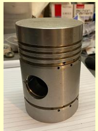
Southern Cross diesel piston. All grooves, seeps and chamfers machined in a powerful lathe with the one groove block, at the same time!
